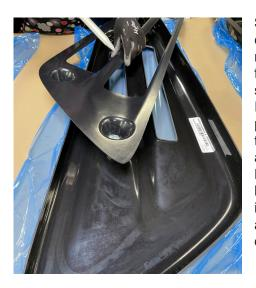
scigrip 400LSE is a two-component (10:1), translucent, methyl methacrylate adhesive for bonding polyolefins with no surface preparation required. It bonds polypropylene, polyethylene and has the ability to cross-bond to metals like aluminium and stainless steel. Product is non sagging, and has short fixture times, making it an excellent choice for assembly and other fabrication or manufacturing uses.
